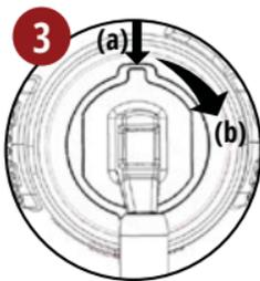
Align (a) plunger stem tabs to slots on valve plunger. Rotate (b) stem to lock. Gauge will face front
