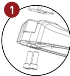
Bolt base & lever assembly together firmly
