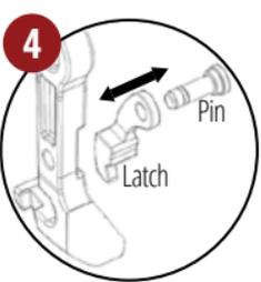
Disassemble 3-piece lever hook, lower and attach to stem, & reinsert the latch & pin to lock hook to stem
