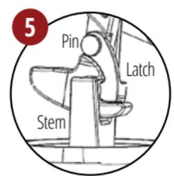
Assembled lever hook will enclose stem & lock in place. Latch will fit into notches on opposite sides of hook
