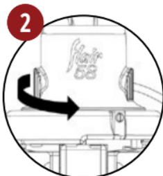
Remove preheat cap & install brew cylinder onto brew base. Rotate counterclockwise to lock
