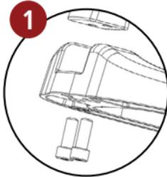
Bolt base & lever assembly together firmly
