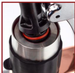
6. Affix gauge and stem by pressing down into the well. Stem should fit flush to top of plunger.
