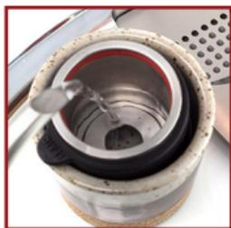
3. Preheat cylinder, with ss plunger inserted, as normal, for at least 30 seconds. This is easiest when brew head is inverted so plunger is on bottom.
